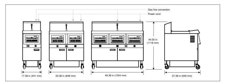
6 burners 255,000 BTU/hr 74.7 kW 1.00 in gas line
