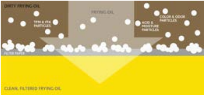
Prime Filter powder attracts and binds impurities in oil, making them too big to pass through filter media.
